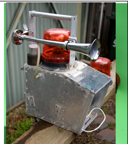
The BHSA automated starting system
